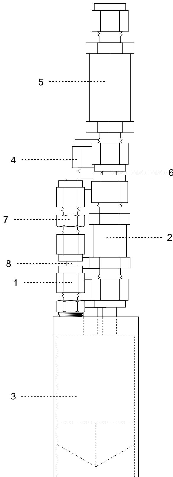
The check valve, SS-CHS4-10, shown as item 2 is available in cracking pressures of 5 psig through 100 psig in 5 psig increments. To be sized properly, the cracking pressure must be greater than the head pressure the pump sees by being placed at different water depths. This is so that the pump will not flood until the vacuum is applied to it. To size the check valve for a particular depth range use : cracking pressure = (max depth +5)/2.3
